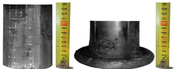
Fig. 20. Lead sample № 11 with size mesh applied to the SR (left) and lead sample № 5 after the research of the SR (right)
