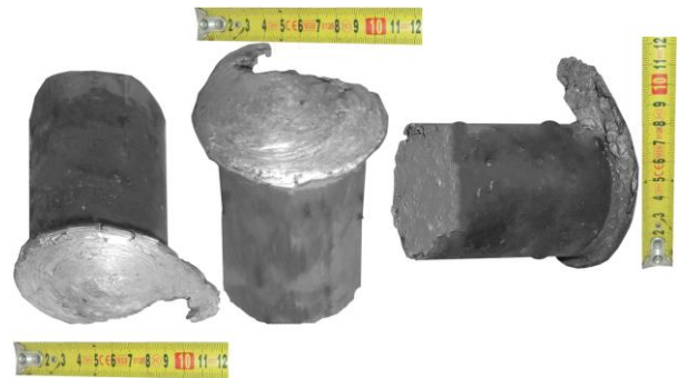
Fig. 23. Sample №12 of aluminum AD 1 after the destruction
