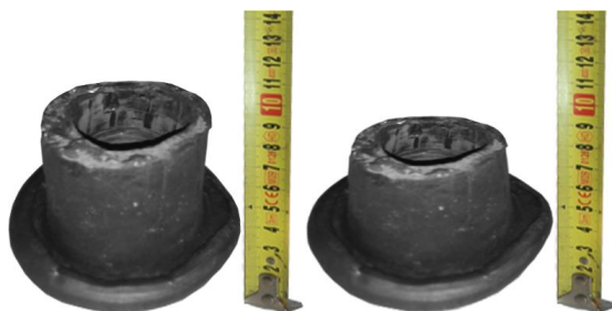
Fig. 19. Plumbum blanks №8 (left) and №6 (right) at intermediate stages on the SR
