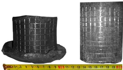
Fig. 22. Sample №11 of aluminum alloy AD 1 before SR (right) and after the destruction (left)
