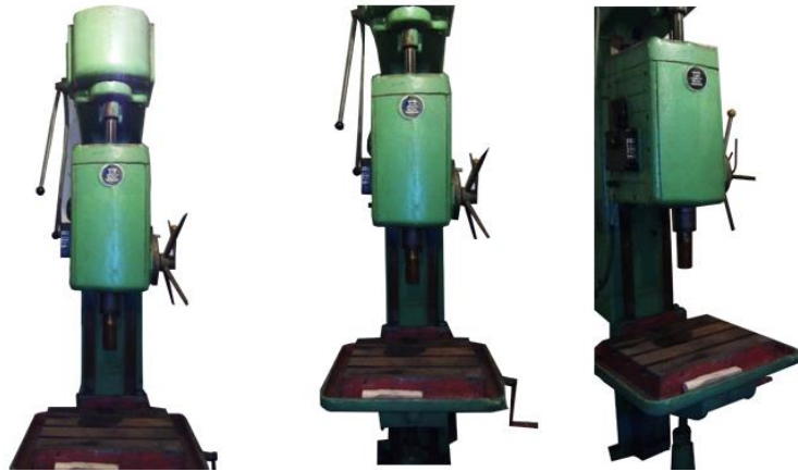
Fig. 1. Vertical-drilling machine 2A-135, to conduct a study of the SR process
