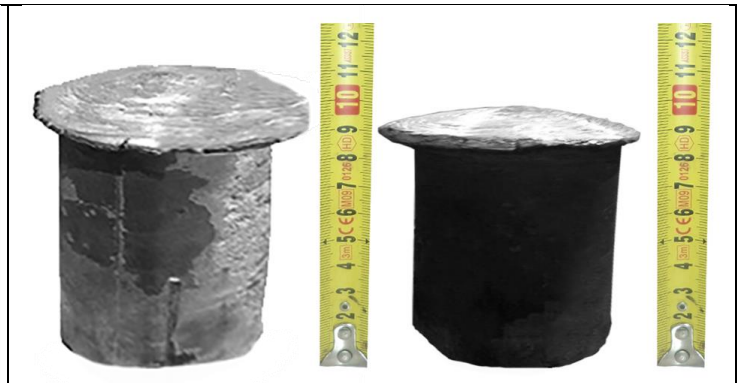
Fig. 11. Cylindrical billets made of aluminum alloy AD 1 after the experiment
