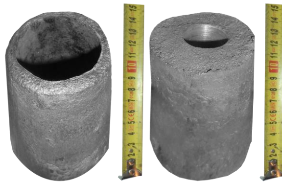
Fig. 12 – Pipe cylindrical billets made of aluminum alloy AD 1 before the experiment
