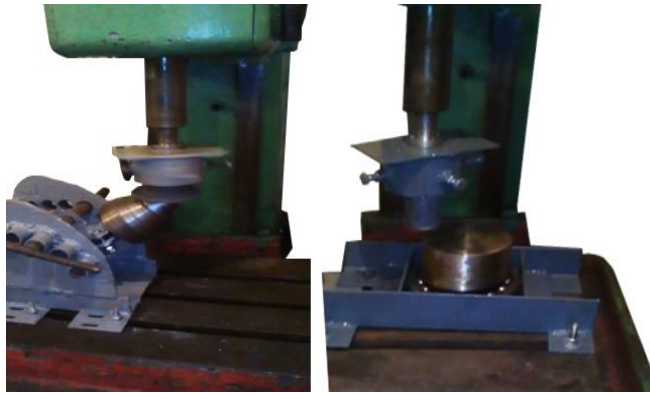
Fig. 15. Pipe, cylindrical billets № 4 (left) on PSR-2 and 10 (right) on PSR-1 prefix, which are made of lead and AD 1 at SR
