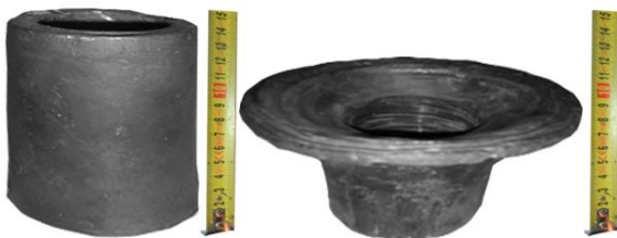
Fig. 16. Plumbum blanks № 8 before the SR (left) and after the research on the SR (right)
