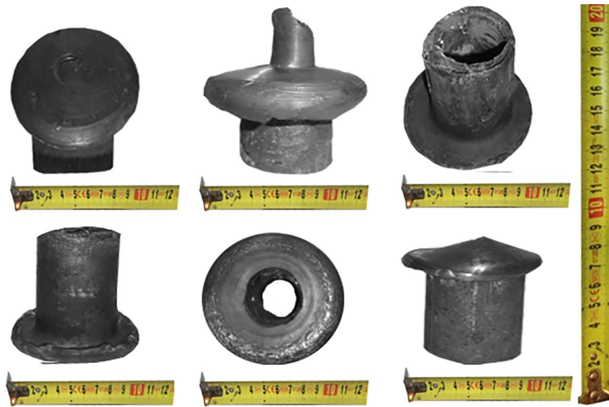
Fig. 21. Plumbum samples №1, 3, 7, 10, 12, 13 after the research on the SR of end
