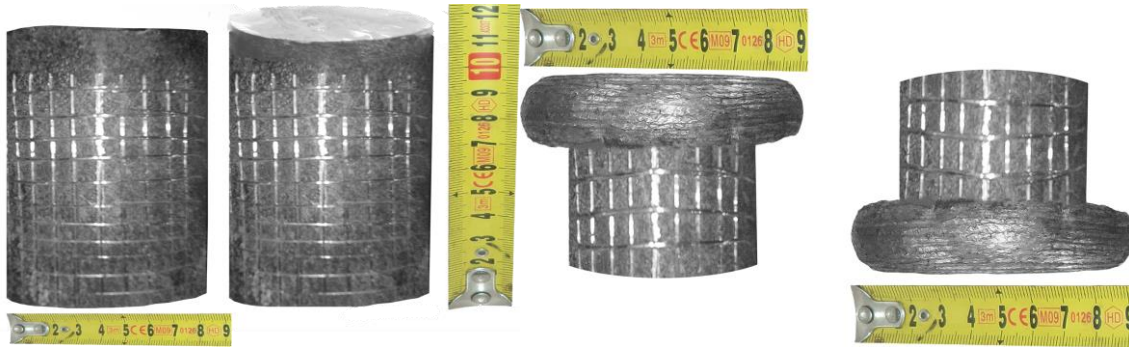
Fig. 24. Cylindrical sample №18 of aluminum alloy AD31T before (up) and after (down) the research on the SR
