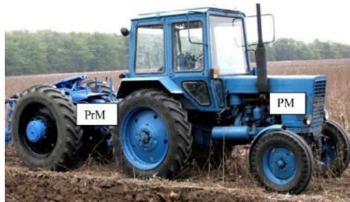
Figure 1. Modular traction vehicle: PM – power module; PrM – process module.
