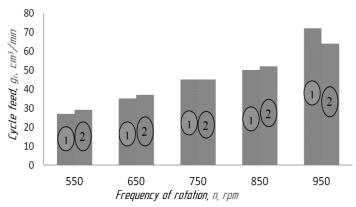
Fig. 12. A graphic representation of the dependence of the fuel supply on the speed of the cam shaft
