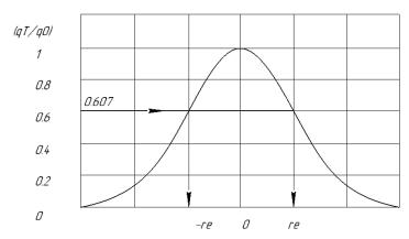
Fig. 6. The scheme for determining the effective value of the jet radius by known irrigation density
