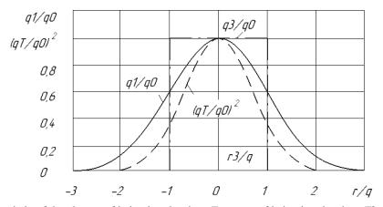
**Fig. 5.** Characteristic of the change of irrigation density qT, square of irrigation density qT2 and equivalent density  $q_e$  related to axial density  $q_o$ .
