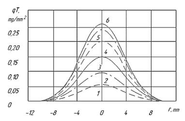
**Fig. 4.** Changing the dispersion of spraying  $q_T$  along the radius of the jet r at a distance of L=50 mm from a spray hole with a diameter d=0.25 mm at injection pressure  $r_{vp}=1.85$  MPa and cycle feed  $g_{ts}=8$  mg at different points in time  $\tau$  from the beginning filing:  $1-\tau=1,026; 2-1,282; 3-1,538; 4-1,795; 5-2.05; 6-2,30.$
