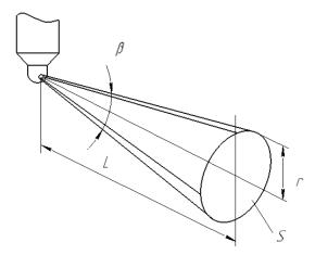
Fig. 3. Geometric characteristics of the fuel jet
