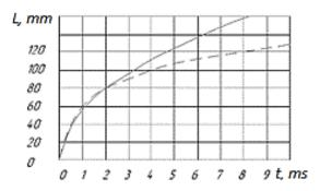
**Fig. 1.** Estimated values of the fuel jet length L: solid line - by the method of A. Lishevsky; intermittent - MADI technique [28], a -  $p_{inj}$ = 26 MPa, p= 0,1 MPa, d = 0,54mm,  $\delta - p_{inj}$ = 26 MPa, p = 1,1 M $\Pi$ a, d = 0,23 mm.
